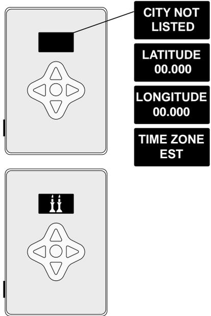
5. Setup is now complete. Make sure to keep your Shabbos Keeper in a proper storage location as described in the installation instructions. To adjust the time, date, or location parameters again, hold down the left and right arrow keys for 5 seconds to reset the device.
